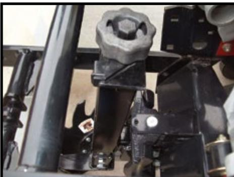
Can be easily adjusted to move trash only or both trash and soil without plugging.
