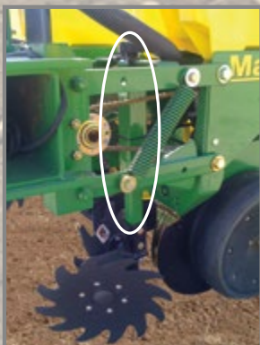
Mounted on JD's screw-adjust conservation tillage hanger bracket
